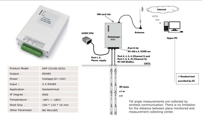
The collector has two independent RS-485 acquisition channels, and expands the external pluggable SD card for data storage and backup. The output supports two communication modes of RS-232 and RS-485, which can be either wired or remote data transmission module, and automatically collect and access data with PC software.
